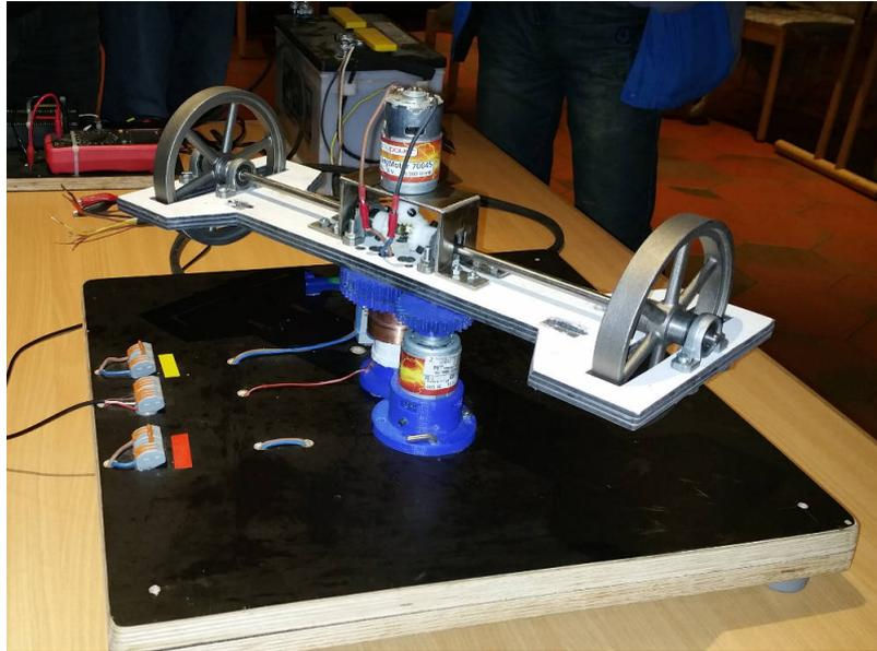
Figure 12: Experimental setup of the double gyro.
